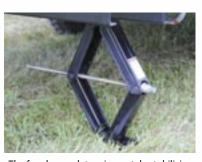
The four heavy duty scissor-style stabilizing jacks extend and retract easily using your cordless drill and provided drill bit.
