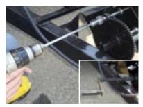
The easy-to-use dual drive winch and drill bit, combined with your cordless drill, raises or lowers the roof in under 30 seconds.
