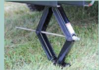
Four standard heavy duty stabilizing jacks
